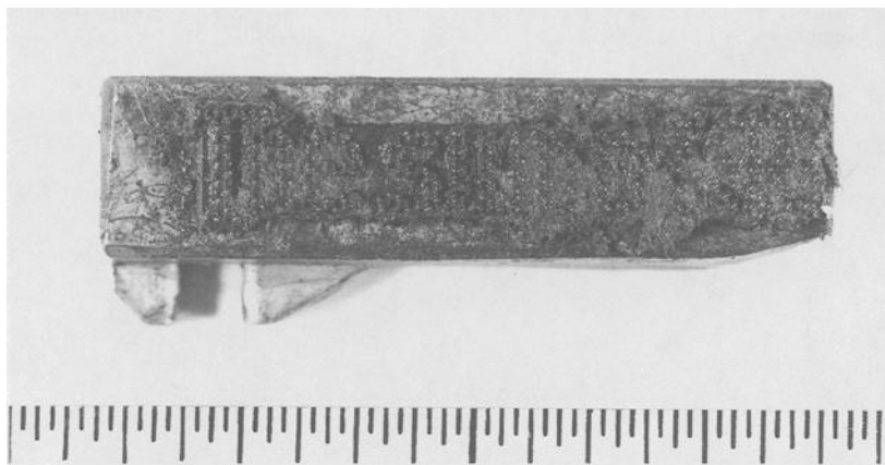
FIG. 3—Slug containing the typeface for "The sum of" prefix (photograph printed backward to facilitate viewing).
